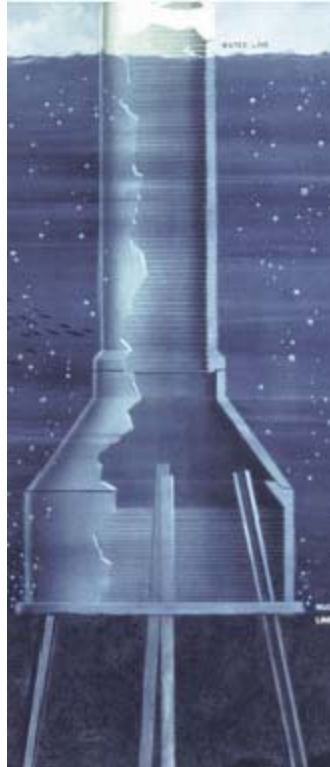
Figure A-12. Use of a precast concrete element as a template for batted H-pile on bridge pier for the Richmond–San Rafael Bridge, California.
