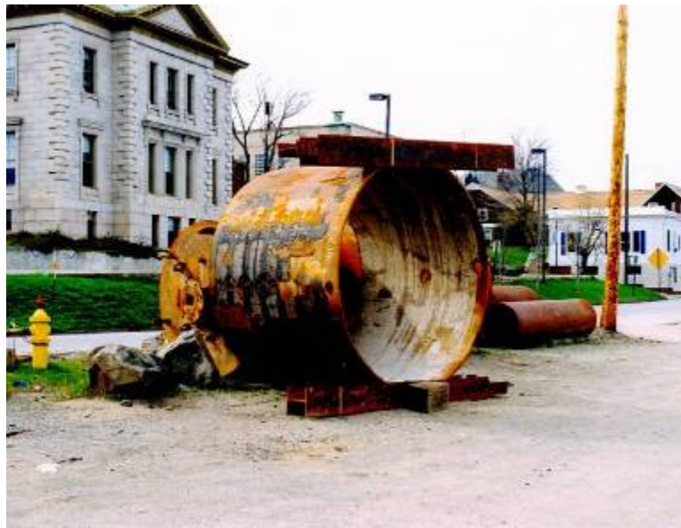
Figure A-34. Sliding upper guide used at Bath-Woolwich Bridge.
