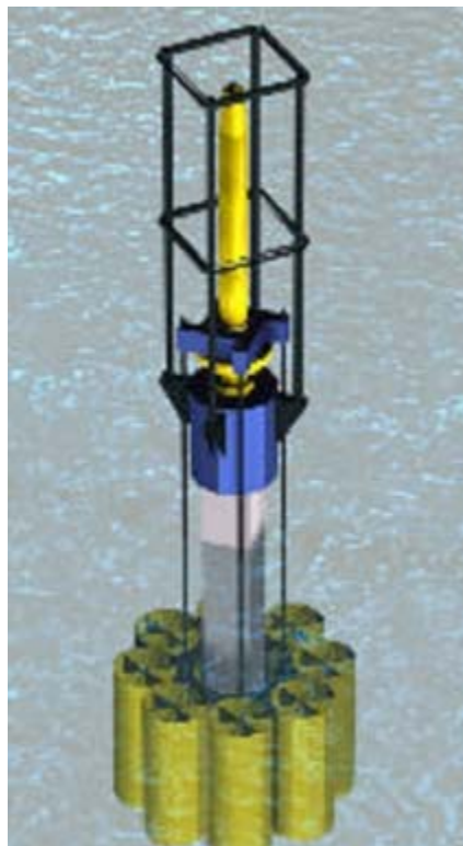
Figure A-53. How water can be used as a counterweight for an over-water statnastics test.
