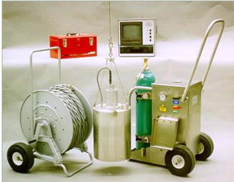
Figure A-123. Shaft Inspection Device (SID).
