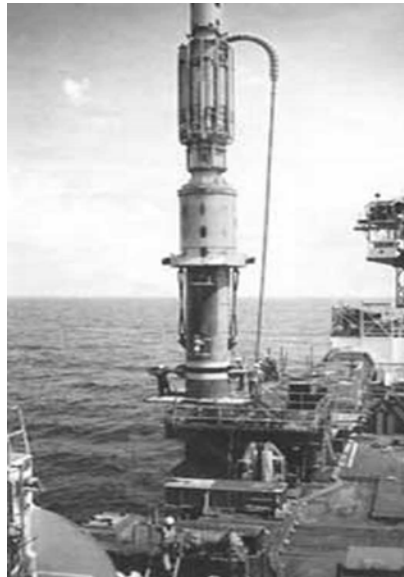
Figure A-48. Menck 500T underwater hammer (after Menck 1999).
