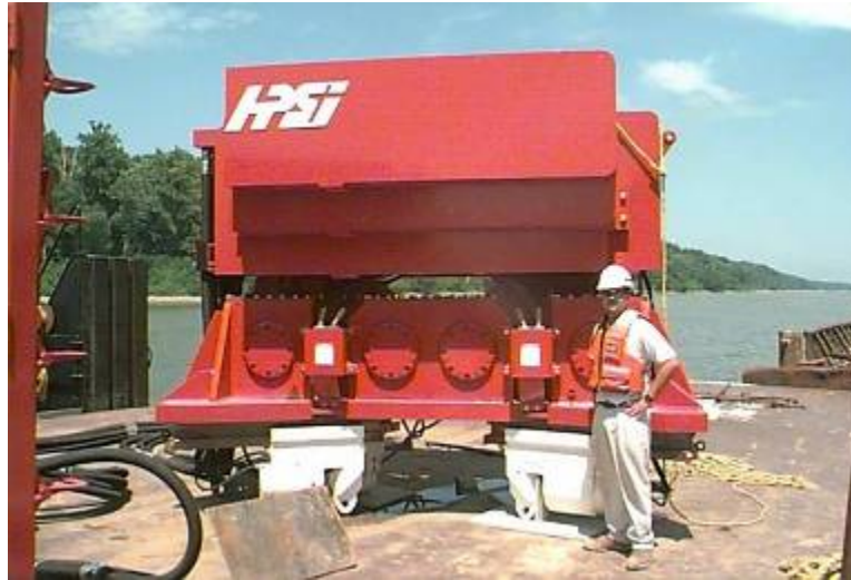
Figure A-64. HPSI Model 2000 vibratory hammer.
