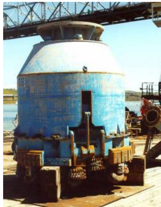
Figure A-45. Under-reamer bit with 10-foot diameter used on the drilled shafts on the New Carquinez Bridge.
