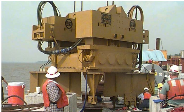
Figure A-66. King Kong APE vibratory hammer.
