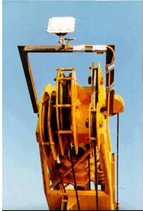
Figure A-106. GPS target sensor on crane boom.
