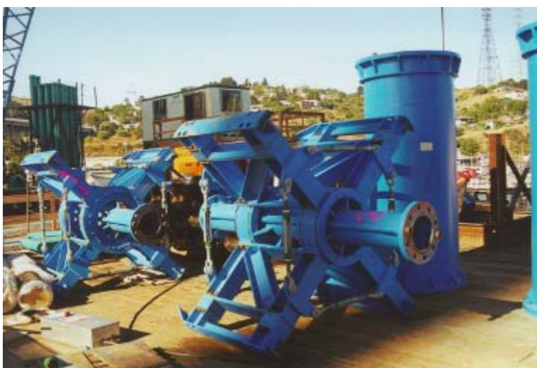
Figure A-47. Centralizers used on the drill string at the New Carquinez Bridge.
