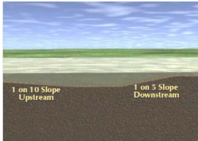
Figure A-73. Basic dredging profile.
